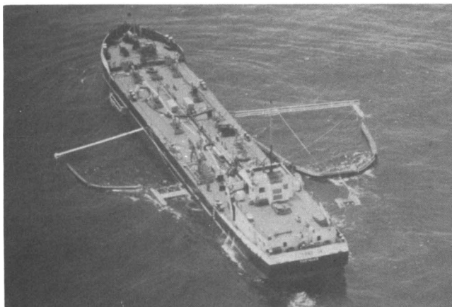
Figure 7. Coastal oil tanker equipped with Sirene 20 and ESCA recovery devices
