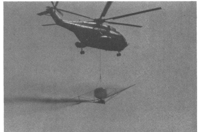
Figure 9. Heavy helicopter (Super-Frelon) equipped with dispersant spraying equipment
