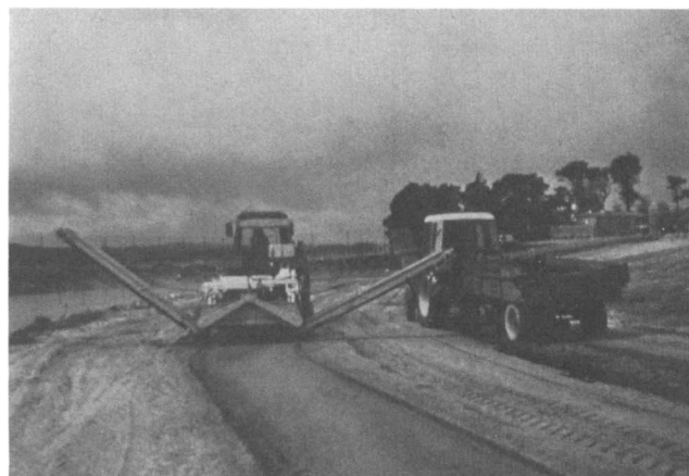
Figure 13. Rolba—adapted screening machine for beach cleaning
