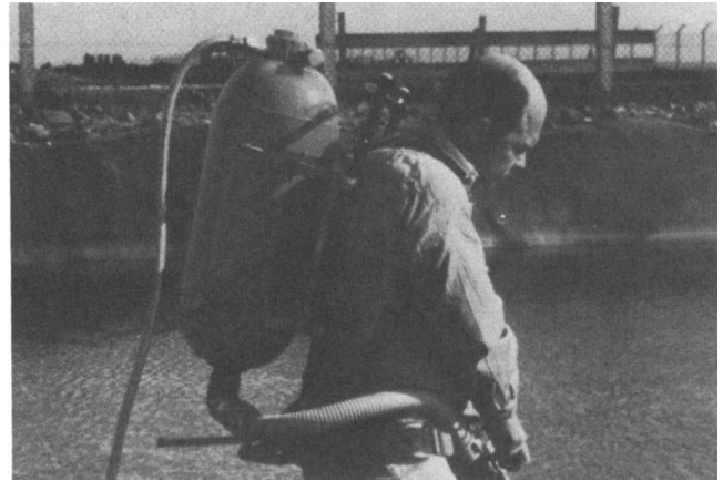
Figure 16. Portable vacuum tank VIP
