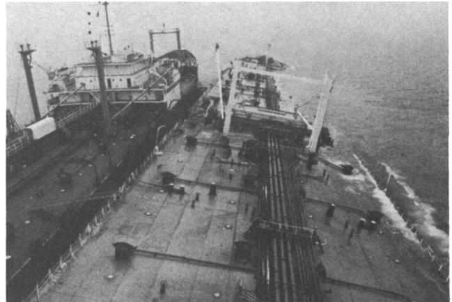
Figure 4. Lightening of a vessel in difficulty
