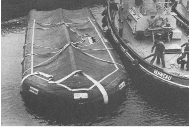
Figure 6. The flexible floating tank, Pollutank
